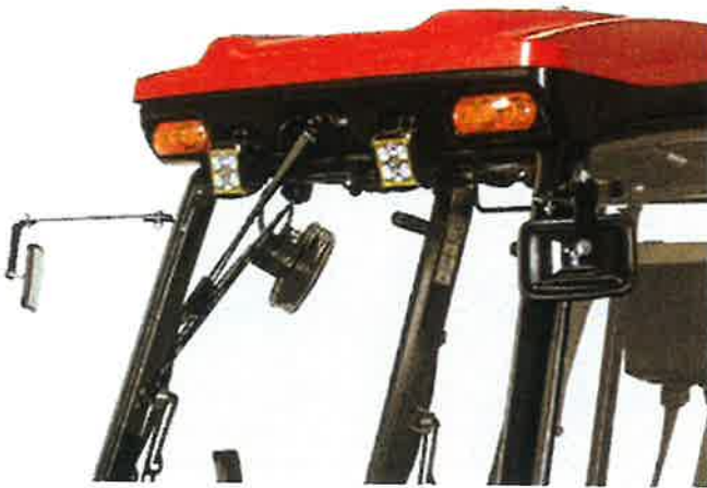
LED Work Lights, 2 Front and 1 Rear
