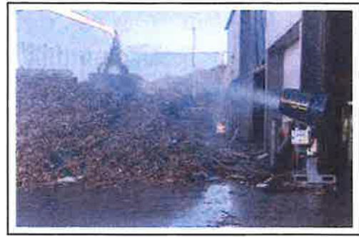
View 5: Screenpod S45 Dust Cannon in Operation
