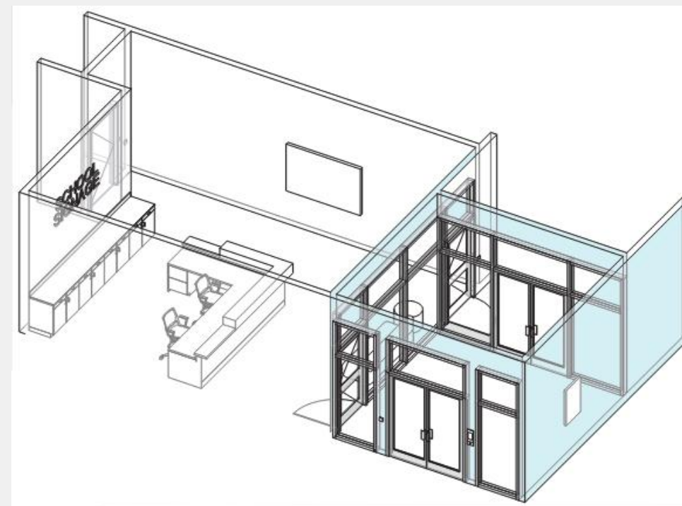
CISD Design Guidelines - Typical Secure Vestibule Upgrade
