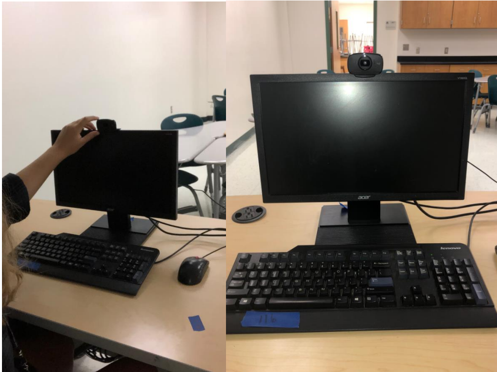
ACISD Summer Workers installing new webcams on all teacher computers. We tested these out and they provide good picture and sound. The cameras have a 360 degree turn radius so the camera can be pointed anywhere in the room.
