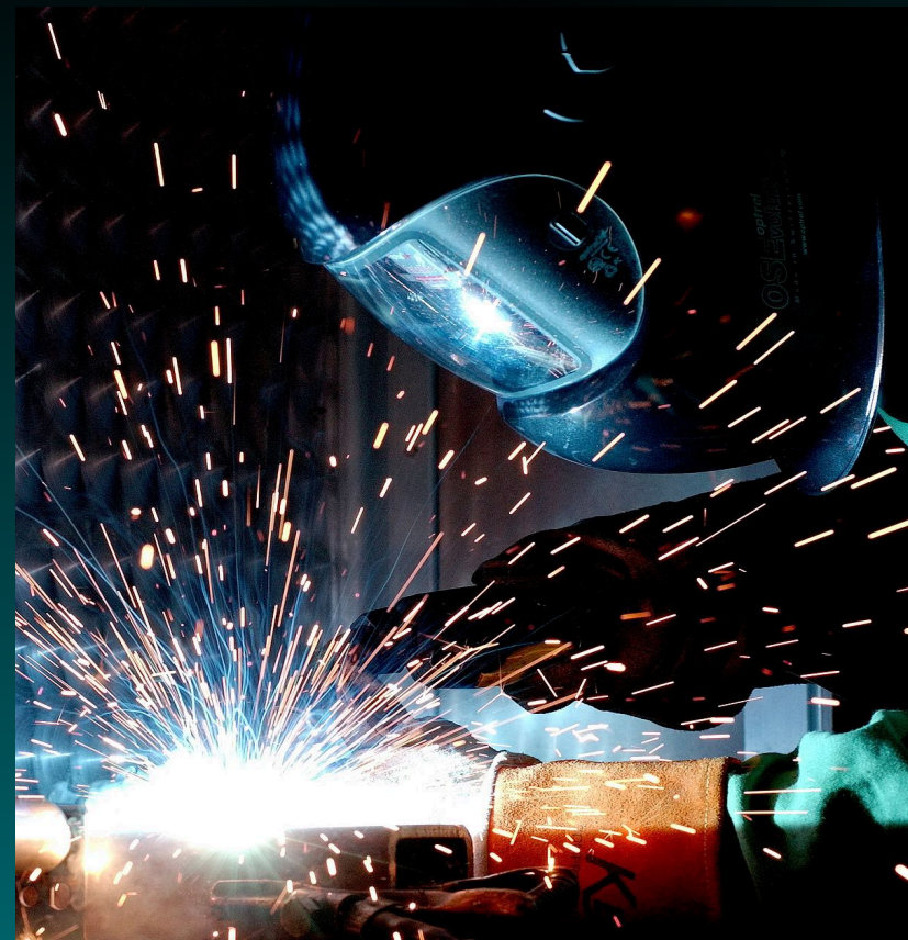
Gas Metal Arc Welding
