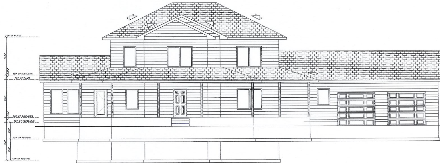
FRONT ELEVATION SCALE: 1/4" = 1'-0"
