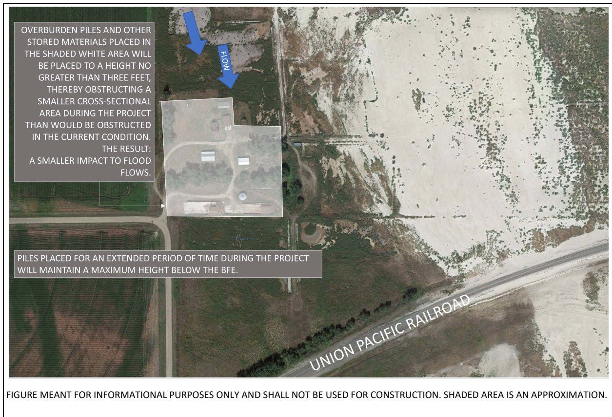
Figure 3: No-Rise area wherein excavated materials replace existing structures
