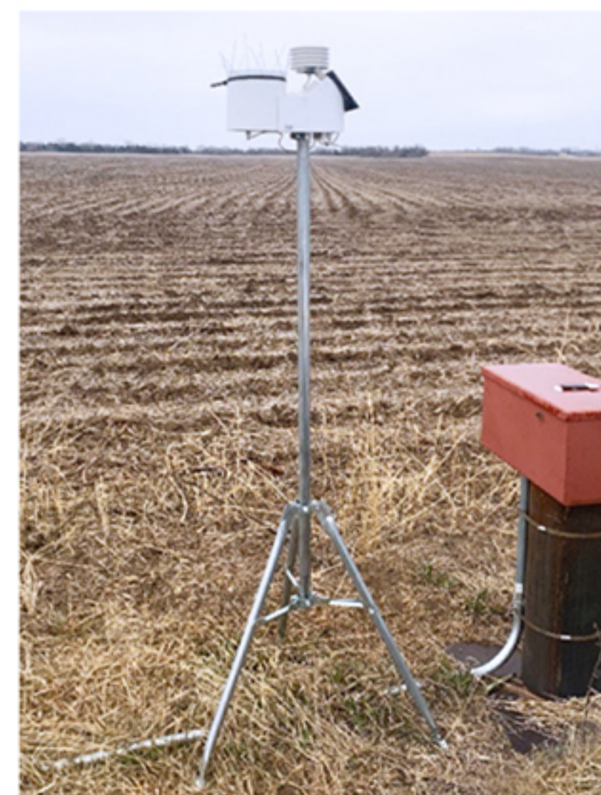
Weather station positioned alongside a monitoring well.
